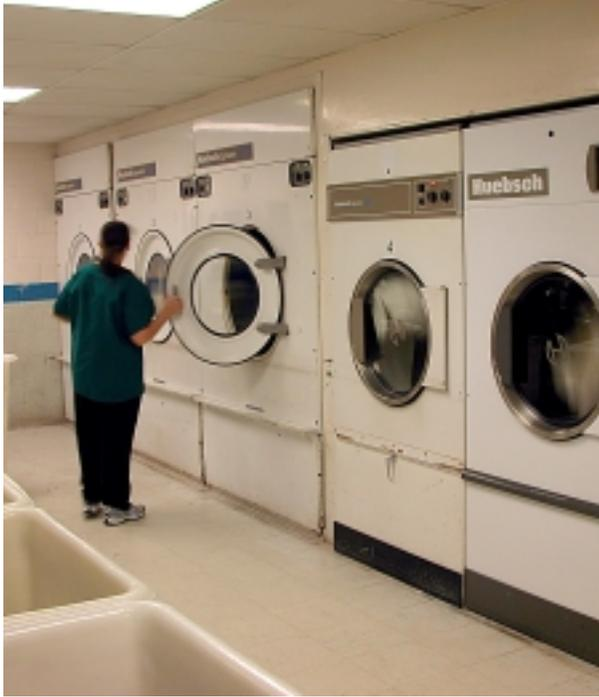
Increases efficiency and reduces energy by automatically adjusting exhaust based on the number of dryers in use.
