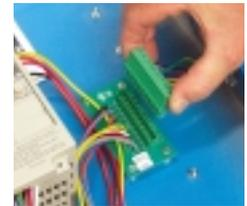
*Wiring harness facilitates field wiring and correct connections.*
